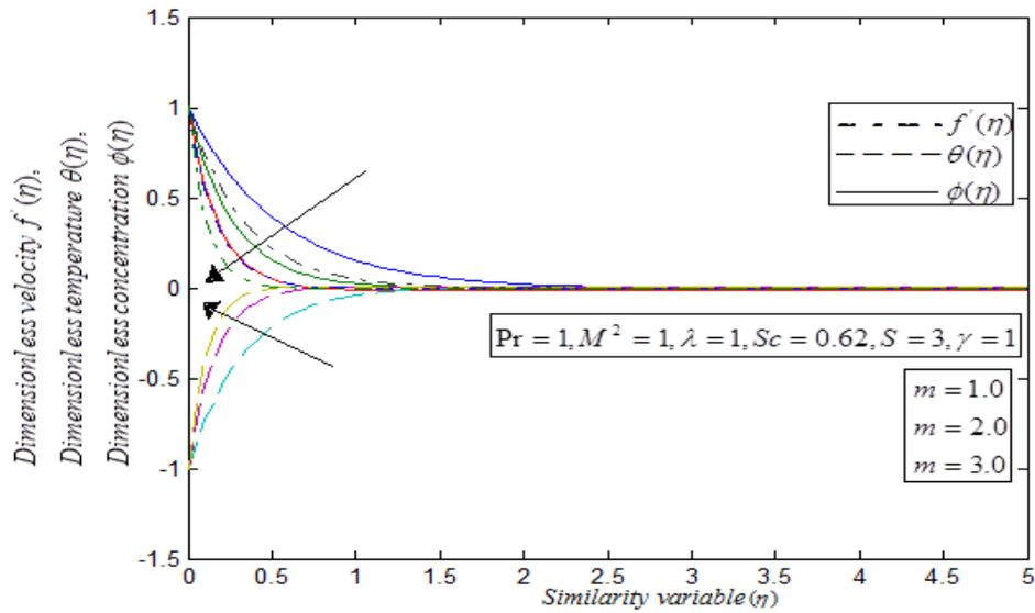
**Fig. 5:** Dimensionless velocity  $f'(\eta)$ , dimensionless temperature  $\theta(\eta)$  and dimensionless concentration  $\phi(\eta)$  versus the Similarity variable  $\eta$ . The curves are plotted for various values of the skin friction  $m$  and some fixed values of the other parameter  $Pr, \lambda, Sc, M^2, S, \gamma$  using the eqns. (20), (21) and (22), when  $h = -0.0066$
