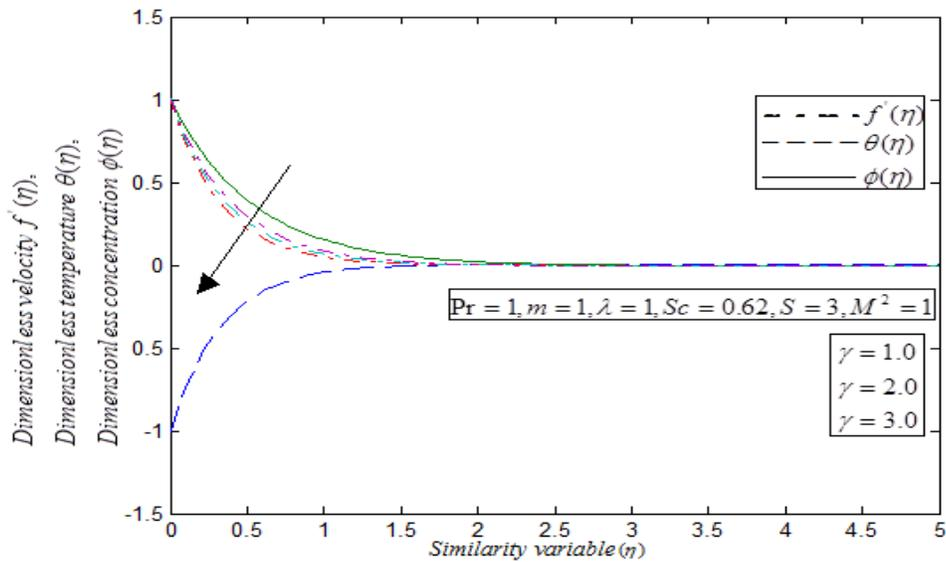
**Fig. 3:** Dimensionless velocity  $f'(\eta)$ , dimensionless temperature  $\theta(\eta)$  and dimensionless concentration  $\phi(\eta)$  versus the Similarity variable  $\eta$ . The curves are plotted for various values of the chemical reaction parameter  $\gamma$  and some fixed values of the other parameter  $Pr, \lambda, Sc, S, m, M^2$  using the eqns. (20), (21) and (22), when  $h = -0.00362$ .
