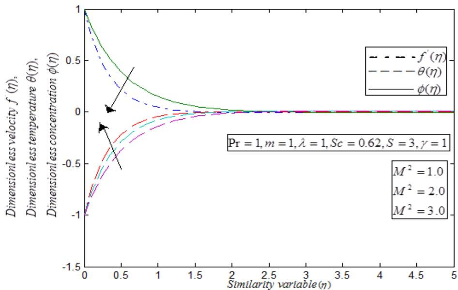
**Fig. 4:** Dimensionless velocity  $f'(\eta)$ , dimensionless temperature  $\theta(\eta)$  and dimensionless concentration  $\phi(\eta)$  versus the Similarity variable  $\eta$ . The curves are plotted for various values of the magnetic parameter  $M^2$  and some fixed values of the other parameter  $Pr, \lambda, Sc, m, S, \gamma$  using the eqns. (20), (21) and (22), when  $h = -0.0066$ .
