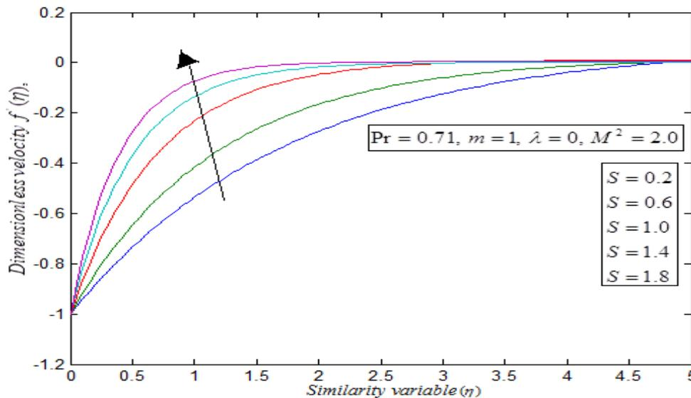
**Fig. 2:** Dimensionless velocity  $f'(\eta)$  versus the Similarity variable  $\eta$ . The curves are plotted for various values of the suction parameter  $S$  and some fixed values of the other parameter  $Pr, \lambda, m, M^2$  using the eqn. (20), when  $h = -0.0067$ .
